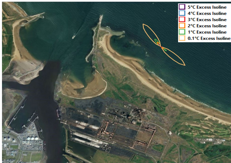
Figure 10. CORMIX excess temperature isolines (°C) under mean spring, peak flood (SE) and ebb (NW) tidal states
